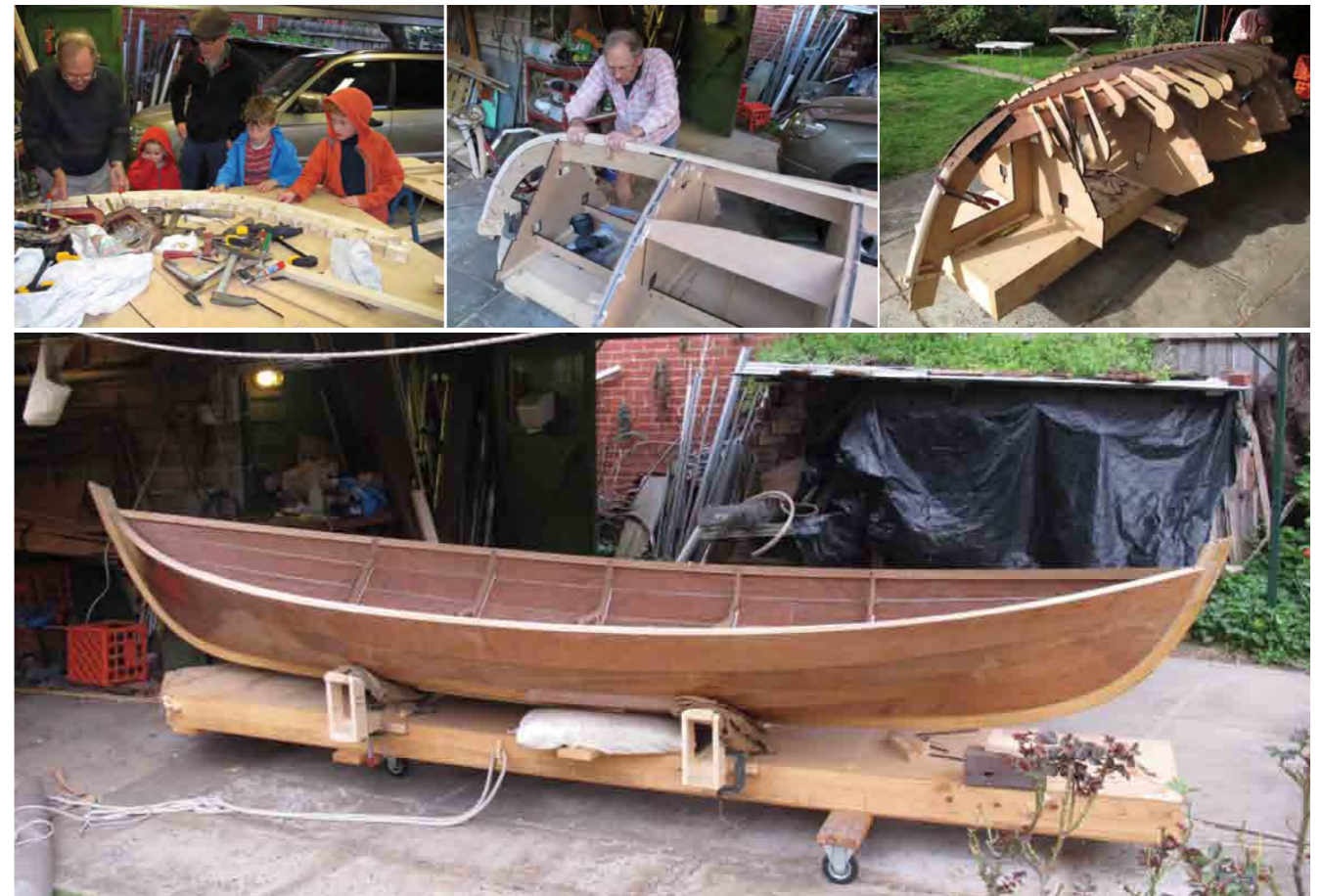
TOP L-R: Making stems for Wemyss Skiff, three generations of Stamps at work here; And ... they fit! ... Wedge clamps holding planks in place without screws.
